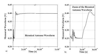
Fig. 6. TDR waveform of the biconical antenna for a 100 ns-long time window a), zoom of the initial portion of the waveform b).
