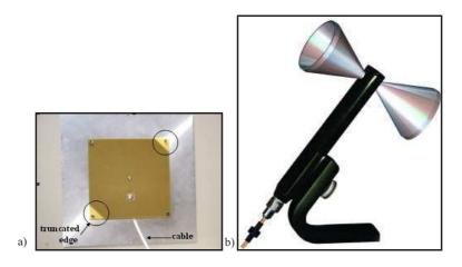
Fig. 1. RFID-reader antenna a), and biconical antenna b).
