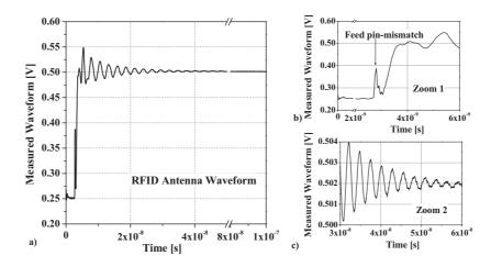
Fig. 3. TDR waveform of the RFID antenna for a 100 ns-long time window a), zoom of the initial portion of the waveform b), zoom of the noise-corrupted multiple reflection at longer times c).
