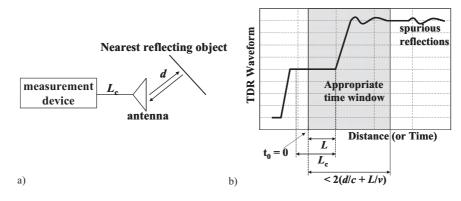
Fig. 2. Schematization of possible interferences from the environment a), and of the corresponding TDR waveform b).
