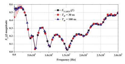
Fig. 7. Comparison between  $S_{11,REF}(f)$  and the  $S_{11}(f)$  curves obtained from FD-transformed data for different time windows  $(T_W)$ , for the biconical antenna.
